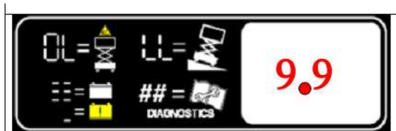
Display screen of the platform control box
